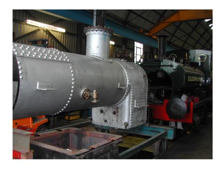
We moved on into the shed, where ex-GWR 4561 was being re-built, although as Ryan said, 85% of what we saw was new - the engine having been in a bad state, having been modified and 'repaired' several times in its life.
