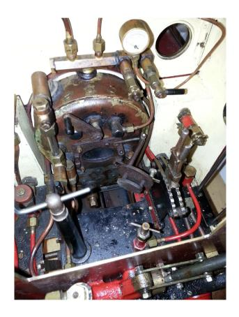
I first removed the cab sides and rear bunker, then the hand pump. Removing the inner bunker was a bit more difficult as the hand pump pipe-work was connected using bulkhead fittings. These were in the bottom corners and somewhat awkward to access. Things were a bit easier once the inner bunker was removed and the remaining pipes either removed or loosened.
